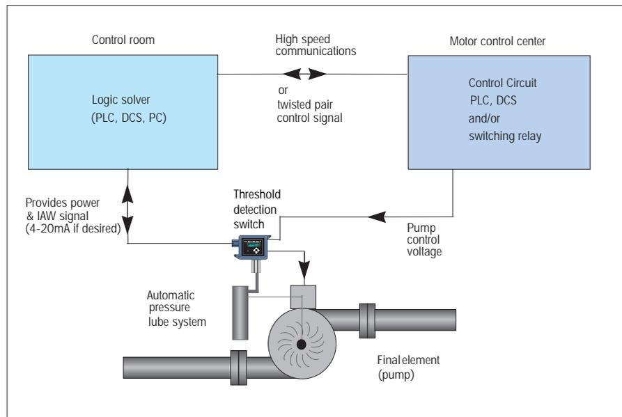
ity, high reliability, direct high level (15 A) switching, and rugged construction for Class I Division 2 hazardous areas (See Fig. 2 for photo, Fig. 3 for schematic).
